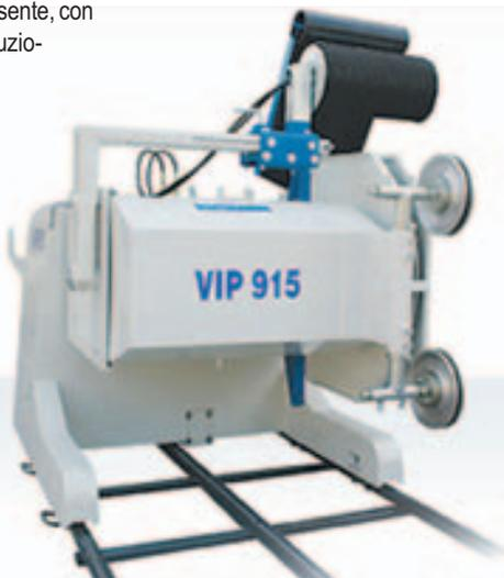
The model with vectorial inverter control system allows to vary the diamond wire speed from 0 to 40 m/sec. in order to optimize its consumption and get the best output, even on very difficult materials. Main electric motor power: 50 - 60 - 75 Hp
