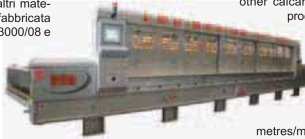
Belt machine used to polish marble and other calcareous materials. It is produced in two versions: KFT 3000/08 and KFT 3000/014, equipped with 8 and 14 spindles, respectively. The max. speed of the mobile beam is 50 metres/minute.
